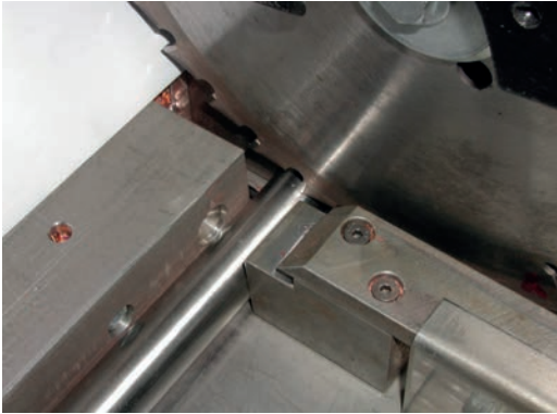
1. Saw off the tubes rectangularly.
