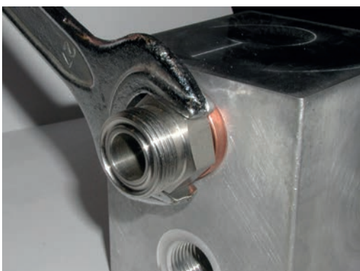
11. Use soft metal seals according to DIN 7603 for sealing the screw-in stub opposite the housing or block.
