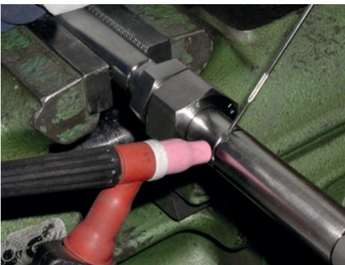
3. Tack-welding when bolted together. Clamping nut slightly tightened. Pay attention to the negative pole.
