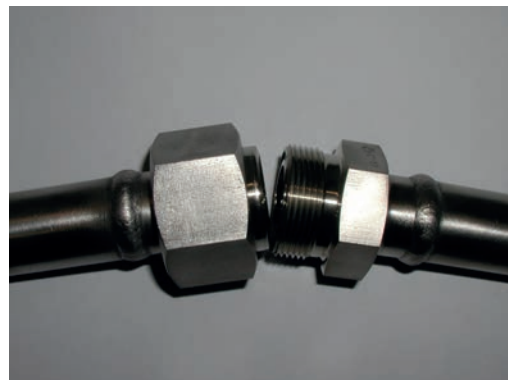
6. Wrong: not properly aligned welded tube union results in leakage
